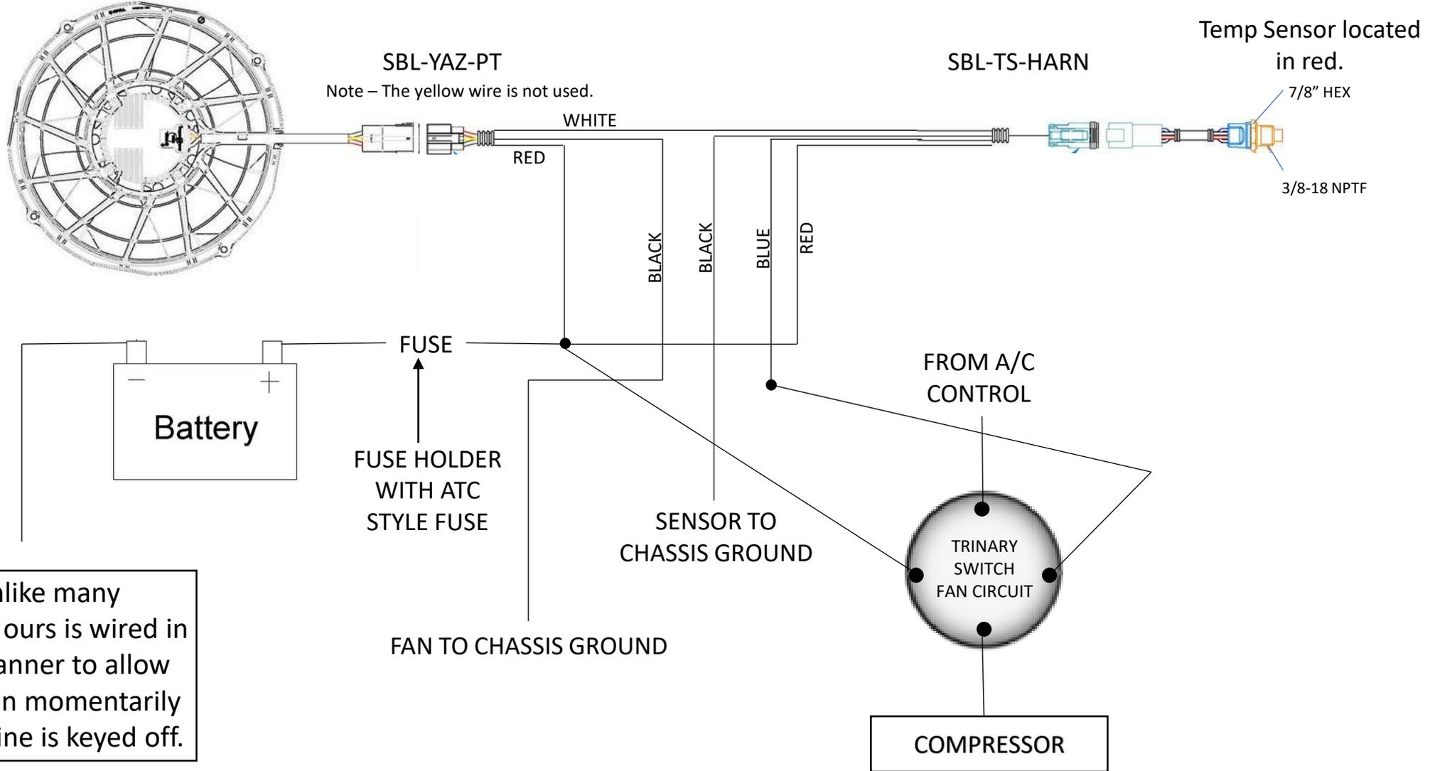
**NOTE:** Unlike many diagrams ours is wired in such a manner to allow fans to run momentarily after engine is keyed off.
